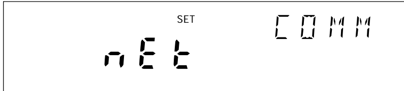
Communications display for setting the network type
