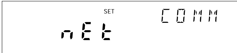
Communications display for setting the network type
