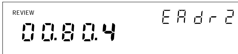
Ethernet address display for viewing byte 2 (for example 00-80- 40 -12-34-56)
